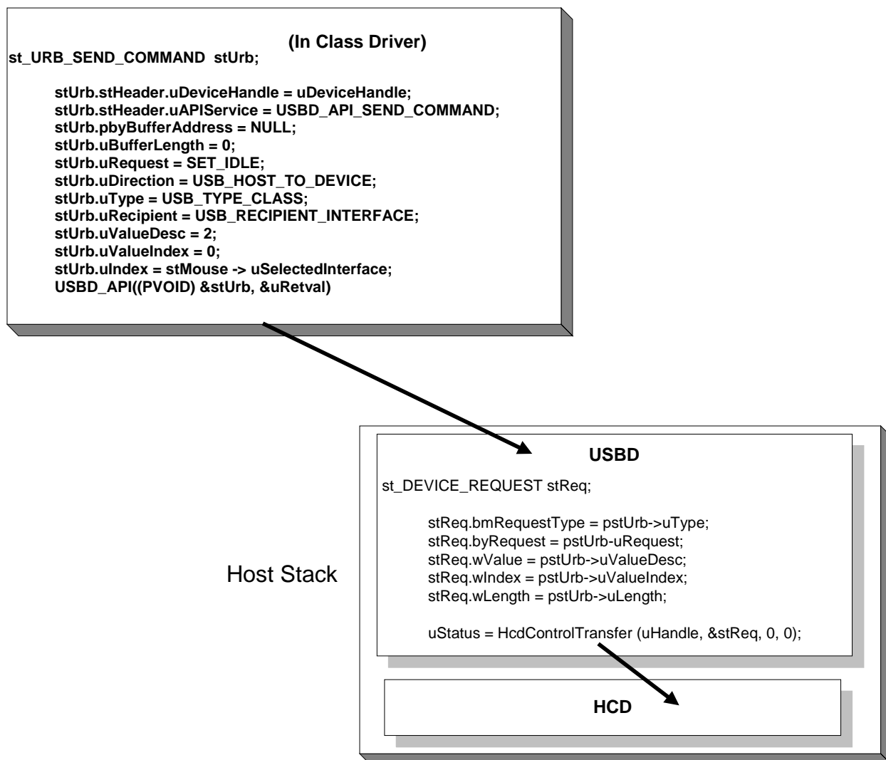
Figure 4-3: Host Stack Calling Sequence Example
